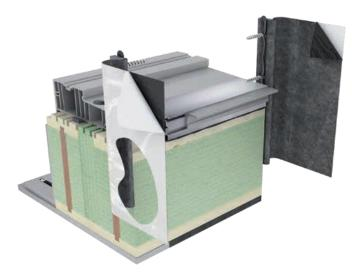
The flange is mounted with at least 4 screws and a glue bead of INSEBO Flanschdicht (in the groove of the plastic strip) in the lower area outside laterally (see illustration).
